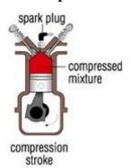
When the piston reaches its lowest limit of travel it then moves upwards, as this happens the inlet valve closes. The exhaust valve remains closed so the cylinder is sealed and nothing can get in or out. As the piston moves upwards the air/fuel mixture (a gas) is compressed to about one
