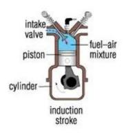
On the induction stroke, the inlet valve opens and the piston, moving down, creates a depression (this is a pressure which is less than atmospheric pressure), a mixture of air/fuel which has become vaporised is pushed into the cylinder via the open inlet valve by atmospheric pressure (a high pressure always flows to a low pressure trying to make pressure equal again).
